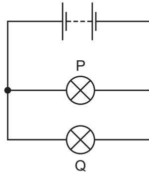
The resistance of lamp Q is larger than the resistance of lamp P.
