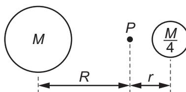
A small mass is placed at point  $P$  such that it experiences zero gravitational force from the masses.
