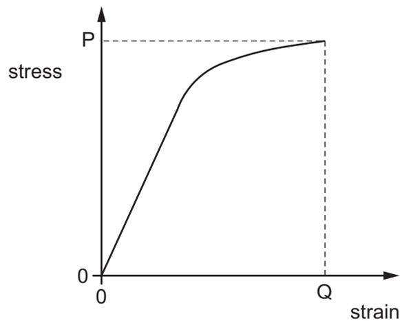
Which feature of the graph gives an indication of the toughness of the material?
