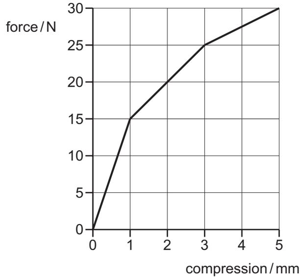
How much energy is stored in the composite spring when the compressive force is 25 N?
